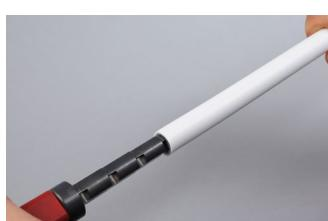
Burr and calibrate the pipe internal surface with the special tool (making sure the cutter and pipe have the same size).
